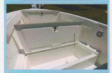
Forward fishboxes provide extra seating and storage area for gear and fish
